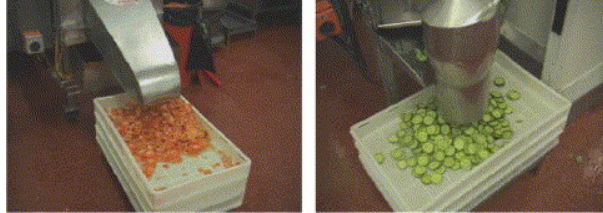
Figure 2.4: Processing fruits and vegetables by " Bernoulli principle " 4
